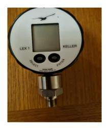
Calibration points for comparison: 900; 950; 1000; 1050; 1100 hPa for increasing pressures/values. Connection ¼" NPT
